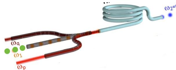
Optimum case: pump 1 velocity matches green signal velocity and pump 2 matches blue signal velocity. Complete collision occurs.
