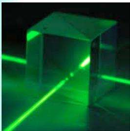
polarizing beam splitter (PBS)
