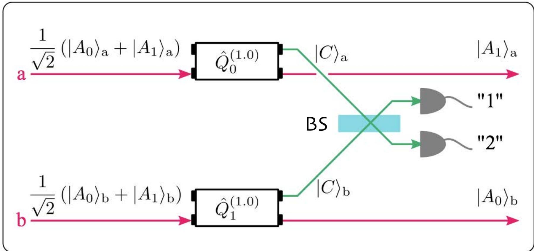
Two TM qubits in spatial beams a and b are fused using two QPGs, which select different "red" TM components and selectively frequency convert them. Then, the "green" outputs of the QPGs are interfered at a 50/50 beamsplitter and detected.
