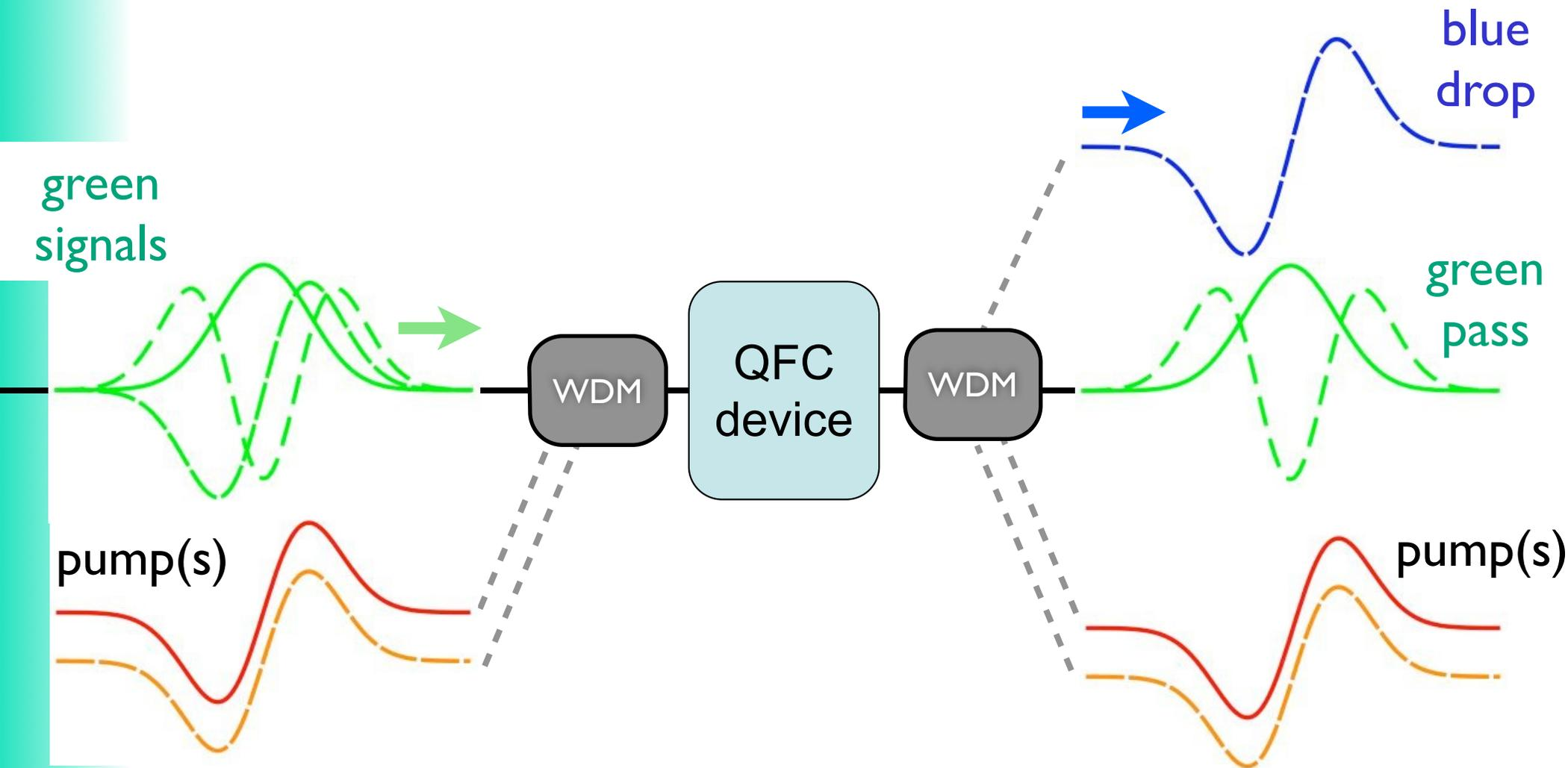
The device is a linear-mode transformer. It treats single-photon packets the same as weak classical (coherent-state) fields.
