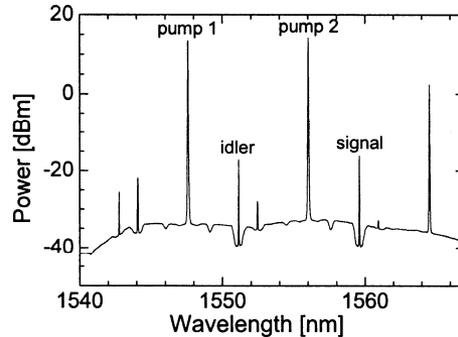
Fig. 2. Example of the optical power spectrum observed at the output of HNL-DSF (Resolution = 0.01 nm).
