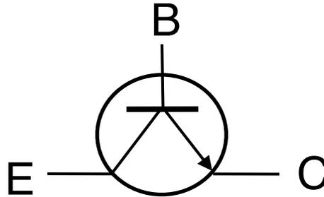
$I_{CE}$  controlled by a small signal on B
