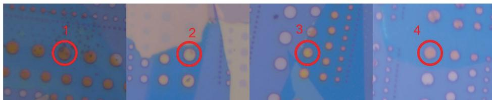
Figure S1. Optical image of the four samples. The pictures were taken after the final SO<sub>2</sub> and NH<sub>3</sub> measurement. Residuals resulting from the two gases can be seen on the surface of sample 1.
