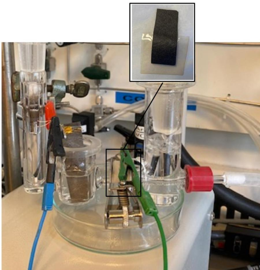
**Figure 3.4:** Experimental setup used for the half-MEA experiments. A glass H-cell with the half-MEA separates the anode and cathode, while the reference electrode chamber is separated by a ceramic frit. The iridium oxide (IrOx) nanoparticles dispersed titanium felt was used as a counter electrode, which remained separate to allow the use of a reference electrode (Hg:HgSO<sub>4</sub>).
