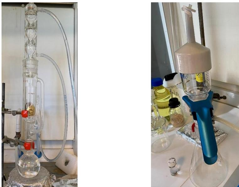
**Figure 3.2:** (left) Soxhlet extractor with Au-coated PCTE membranes. (right) vacuum deposition setup for the catalyst deposition on the metal-coated PCTE membrane.
