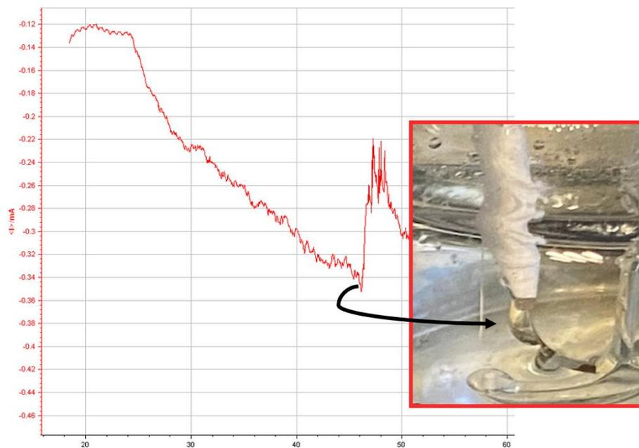
**Figure A.4:** AuFET experiment where a drop accumulates above the electrolyte contact, resulting in increased currents over time due to increased contact of Au to the electrolyte. CA was conducted at  $+0.2 V_{\text{VRHE}}$  with  $\text{O}_2$ -headspace in 1 M  $\text{HClO}_4$  at room temperature.
