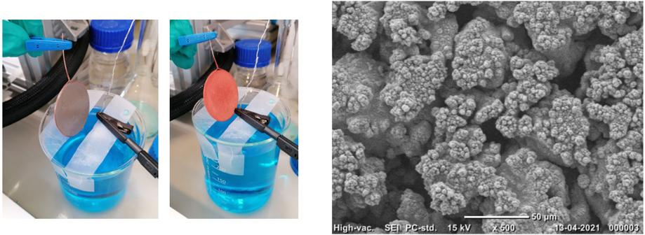
Figure B.18: Electrochemical Cu deposition on porous disk and SEM image of surface morphology. The Cu deposition gives the electrode a red colour and the SEM image shows deposition of small structures.
