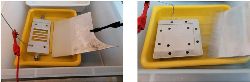
Figure B.6: Electrochemical anodization of aluminium parts for creating a surface protecting layer.
