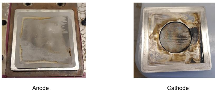
Figure B.14: Reactions of stainless steel with either electrolyte or Li. Thick black deposits on the cathode was observed after a reduction experiment, where also the anode had remnants on its surface. This lead to much colouration of electrolyte (see next figure), probably from iron leaching from the stainless steel.
