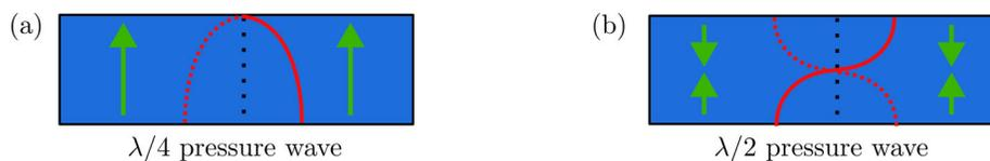
**Figure 4.1:** (a) Standing-pressure  $\lambda/4$ -mode in a microfluidic channel with particles being pushed to the top of the channel (green arrow). (b)  $\lambda/2$ -mode with particle focusing at the channel center.
