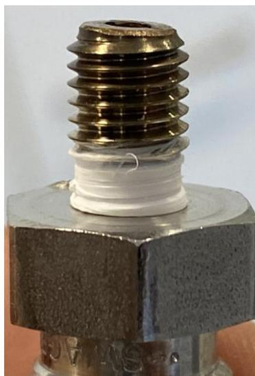
**Figure 3.4:** *Picture of the discoloured Swagelok Part*
