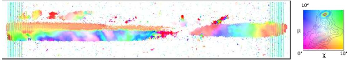
Figure 2.21: A room temperature DFXM mosaicity map and its corresponding pole figure of a deformed grain in highly deformed Fe-Si alloy ( \varepsilon = 2.0 ). The grain slice is illuminated with line beam. The mosaicity scanning is done over 10^\circ in \mu and \chi angles with a step size of 0.5^\circ . Effective pixel size of the map is 400 nm. Courtesy of Can Yıldırım.
