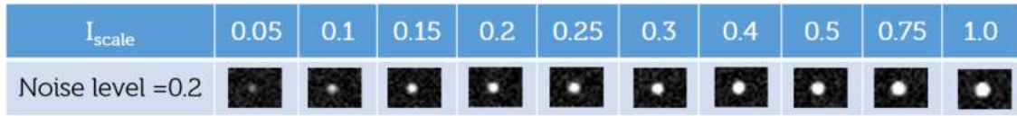
Figure 4.9: The shape change of a randomly chosen ( 1\bar{1}2 ) peak with respect to signal-to-noise variation under noise scaling \alpha = 0.2 condition. For ease of comparison, the contrast setting of all images are set as equal.
