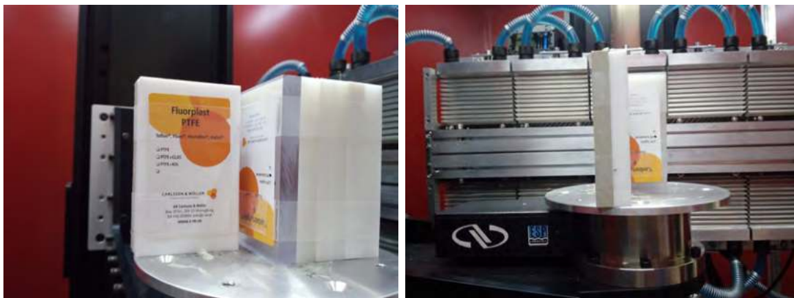
Figure 3.4: Pictures of the sample including seven different plastics, taken from the different angles. The image reconstruction of this sample is shown in Fig. 3.7b.
