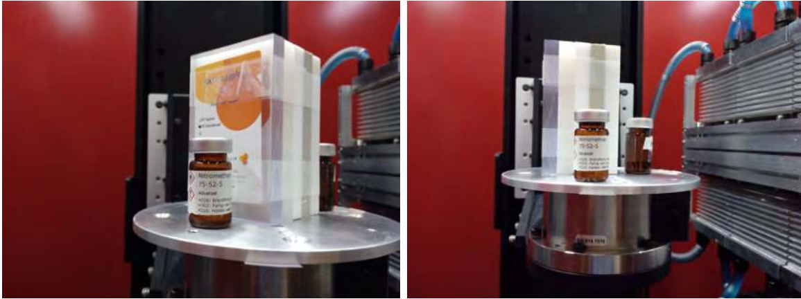
Figure 3.5: Pictures of the sample including five different plastics and the different liquids in two bottles, taken from the different angles.
