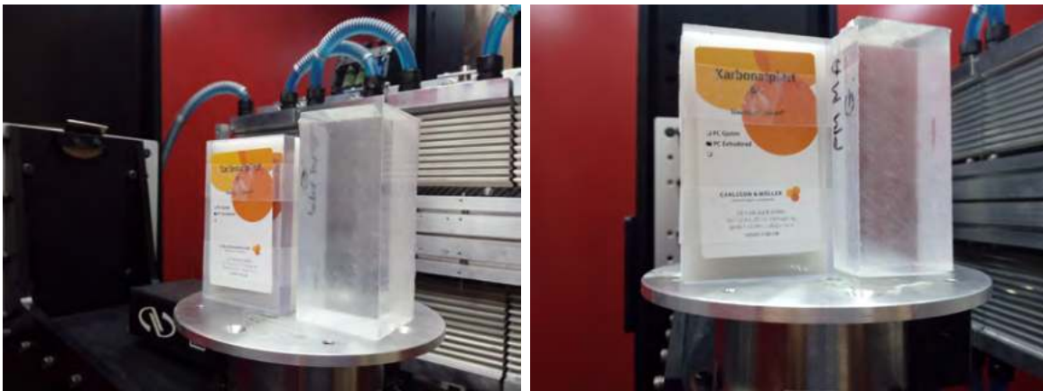
Figure 3.6: Pictures of the sample including five different plastics, taken from the different angles. The image reconstruction of this sample is shown in Fig. 3.7a.
