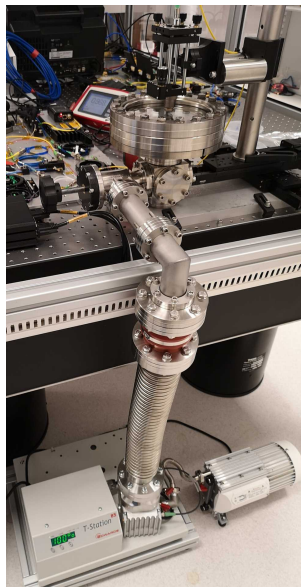
Figure 7.6: Photograph of the setup showing the turbomolecular pump and how it is connected to the vacuum chamber.
