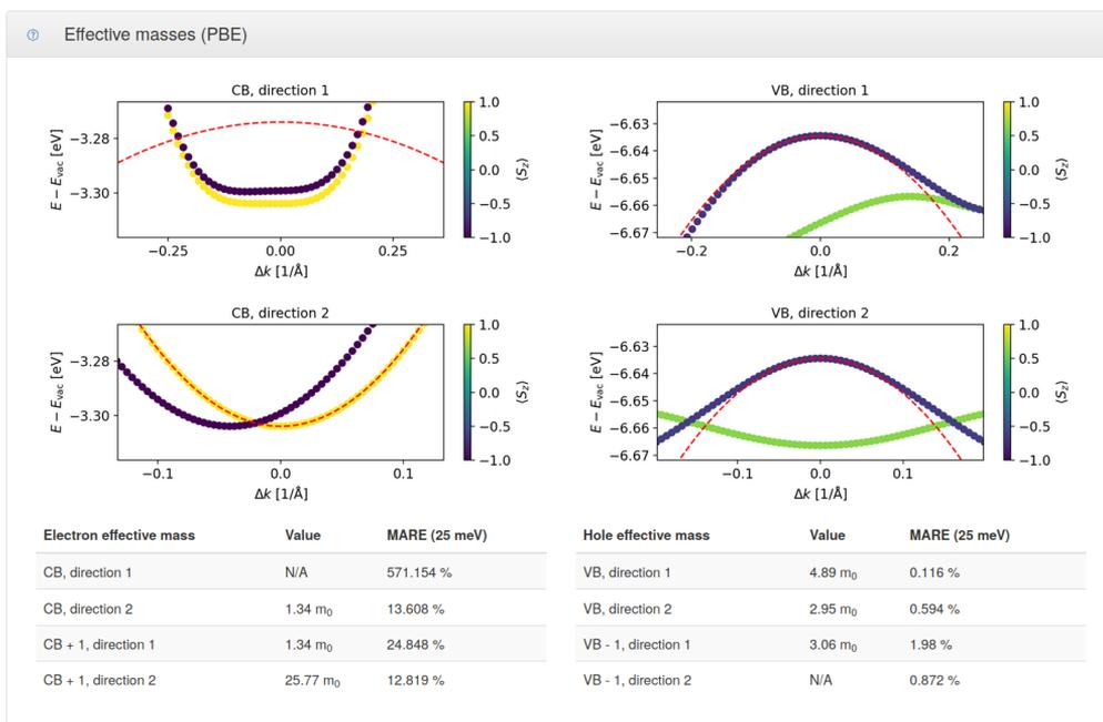
Figure 5.8: Effective mass webpanel for  $\text{BaI}_2$ . Adapted from [66].
