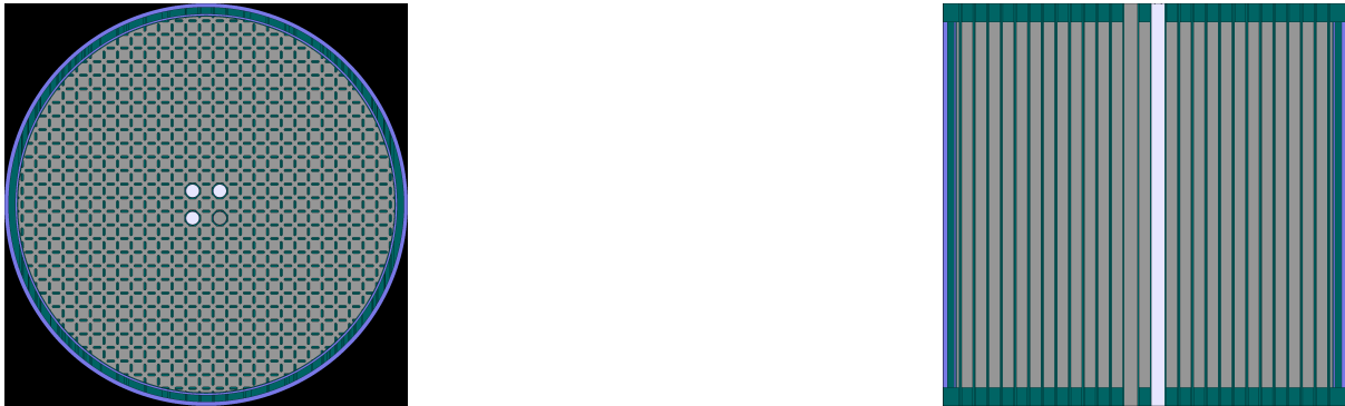
Figure 3.10: MSRE full core model in Serpent: top view (left) and side view (right)
