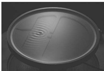
Fig. 1 | The walking droplet double-slit experiment.
